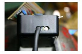
The next few photos show the circuit board with the cables attached, some "tie wraps" (from a local hardware store or home center) put on the cables to strain relief the cables, the circuit board nesting in the box and the final product.
